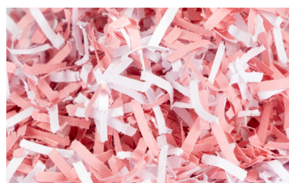
2 x 15 mm particles of security level P-5 according to DIN 66399 (ISO/IEC 21964)
